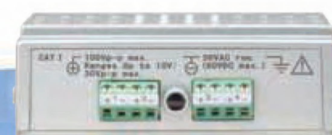
4-channel isolated voltage/temperature terminal unit 4MF
