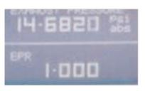
Multifunction, task oriented display readout for up to 4 parameters simultaneously
