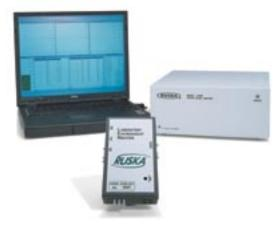
The LEM is compatible with Ruska's Model 2456 Piston Gauge Monitor (PGM) and WinPrompt® software which automates the operation of Ruska's extensive line of primary pressure standards. The LEM allows WinPrompt® to automatically compensate for air buoyancy effects on the mass set of the piston gauge. The LEM is also compatible with the Model 2465 Autofloat Gas Piston Gauge.
