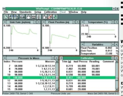
Shown: WinPrompt is acquiring information from the piston gauge through the Piston Gauge Monitor and displaying it in real-time. The data is being used to automatically adjust the pressure/mass values.
