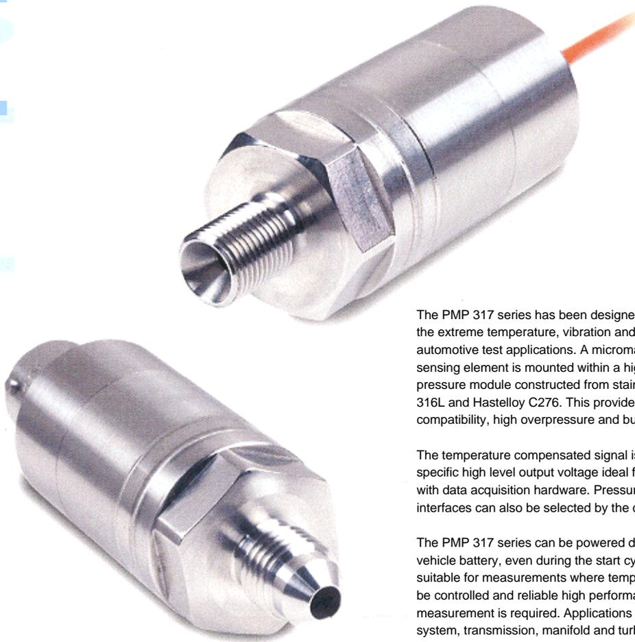
The PMP 317 series has been designed to withstand the extreme temperature, vibration and shock levels of automotive test applications. A micromachined silicon sensing element is mounted within a high integrity pressure module constructed from stainless steel 316L and Hastelloy C276. This provides hostile media compatibility, high overpressure and burst ratings.
