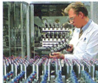
*Computerised testing and calibration of pressure transducers.*
