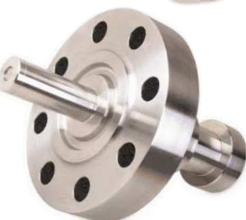
The PTX 400 series of pressure, temperature and combined pressure/temperature transmitters has been specifically designed for long term use in subsea locations. It enables accurate process measurements to be made directly on subsea wellheads and production manifolds. The sensor design is based on API performance requirement PRI and product specification level PSL3.
