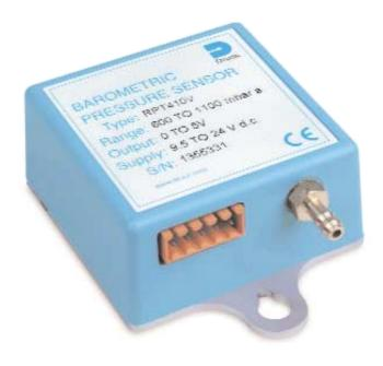
The RPT 410 Resonant Silicon Pressure Transducer (RPT) uses advanced sensor technology proven for highly accurate and stable barometric pressure measurement. For example, Druck RPT technology is used within aircraft cockpits for in-flight air data processing, where the stability of various absolute pressure measurements is paramount.
